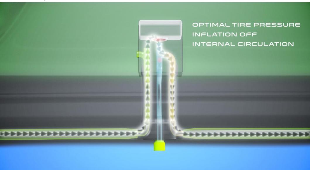
... and it activates internal air circulation when optimal tire pressure is reached.
