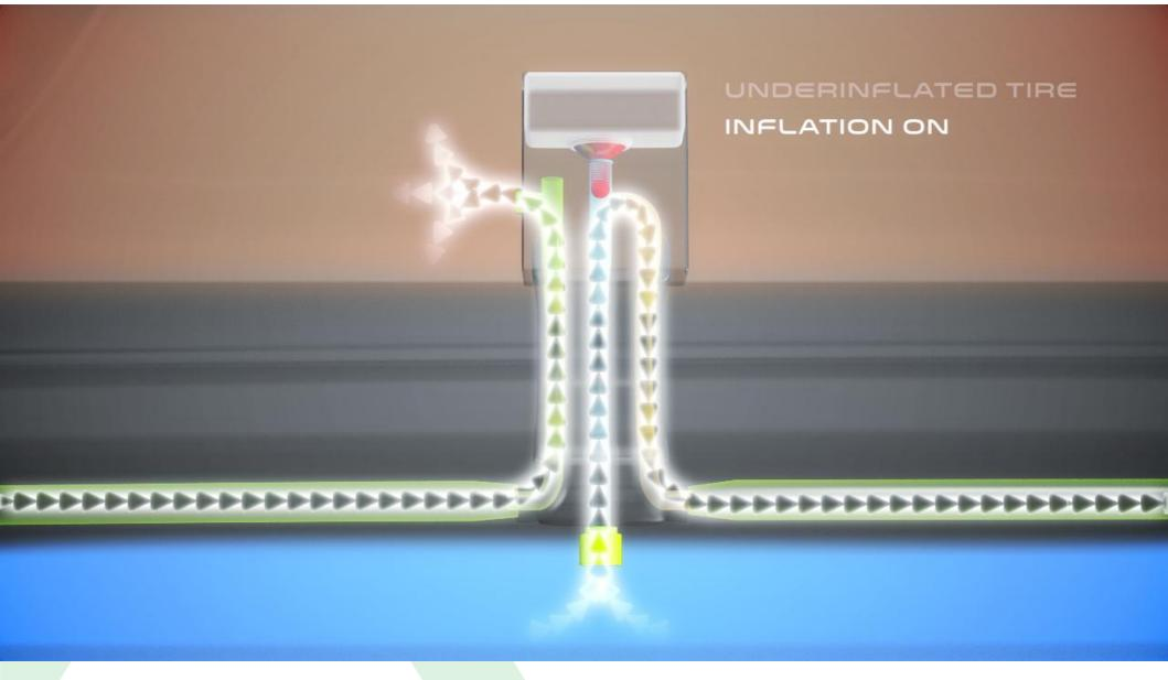
The pressure regulator enables **inflation from outside air** through filter only when needed...
