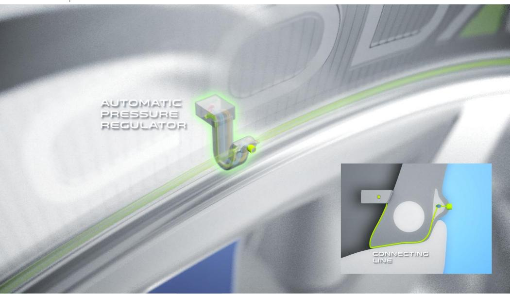
...and an automatic **pressure regulator** with interface connecting the tire interior with outside environment.
