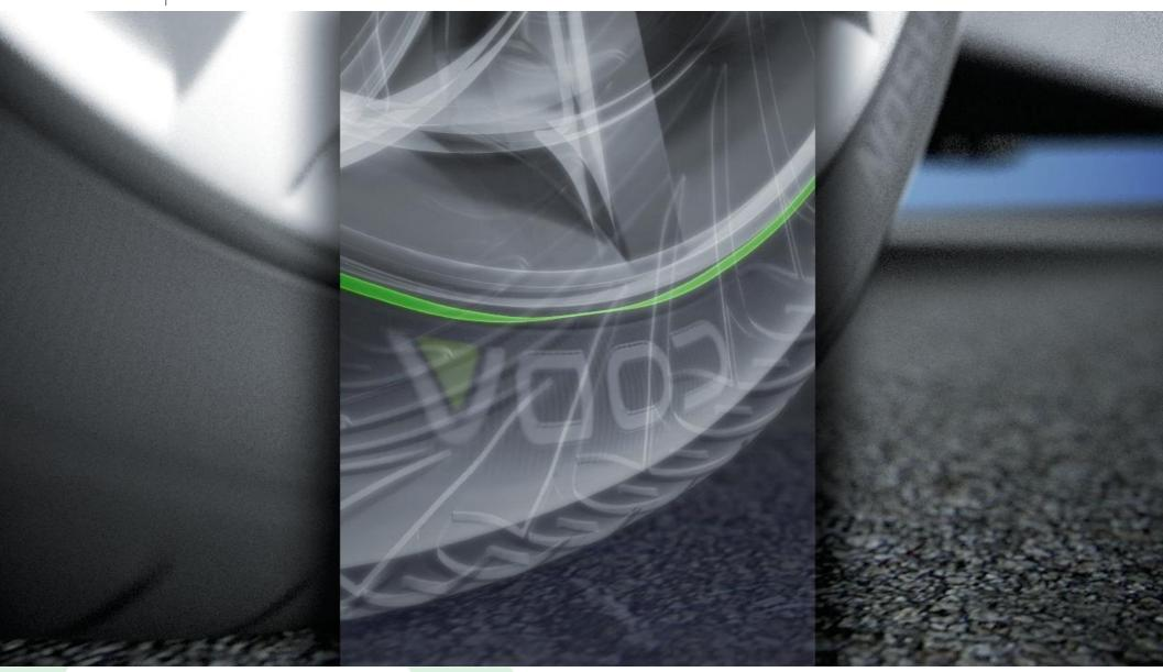
The system integrates a **peristaltic tube chamber into the tire wall**. The chamber is kept **closed at its lowest point** by the normal tire deformation caused by the vehicles weight.
